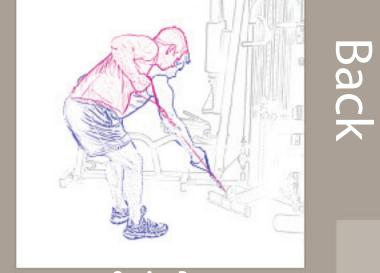
**One Arm Row** Attach the Single Handle to the low pulley. Stand facing the machine, bend slightly at the waist, and grab handle with a neutral grip and pull to midsection **Muscles worked**: Latissimus dorsi, Rhomboids, Trapezius, Deltoids, Forearms, Biceps
