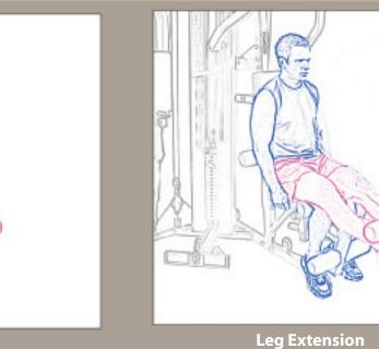
Adjust seat and seat back so that knees are level with and even with pivot point. Sit and hook ankles behind lower roller pads. Extend legs forward and upward. **Muscles worked:** Quadriceps
